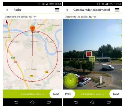
After the endpoint of the link has been aligned, login into the one devices of the link and measure the signal level by using Antenna Alignment and/or perform the Link Test with chosen parameters (duration and packet size):
