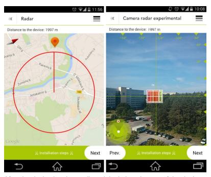
After the device has been aligned, login into the one of the devices of the link and measure the signal level by using Antenna Alignment and/or perform the Link Test with chosen parameters (duration and packet size):
