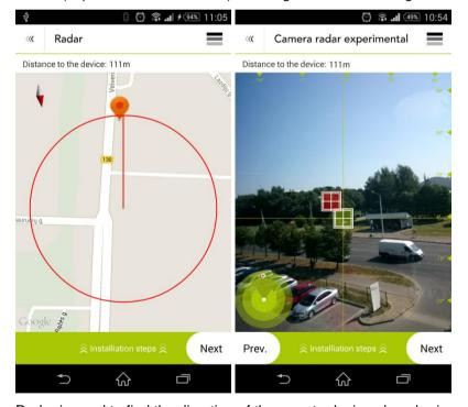
Radar is used to find the direction of the remote device along horizon. Camera radar is used to align and tilt the device.
